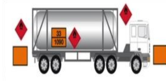
Transport units with a single tank section
