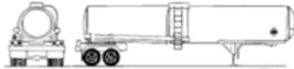
Low pressured chemical tank
